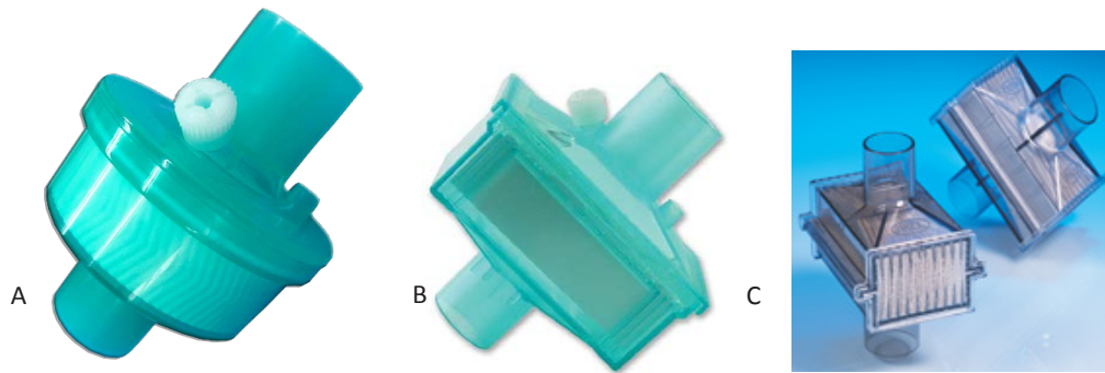
Figure 1 Breathing system filters; heat and moisture exchanger filter (HMEF) (A) electrostatic filter HME, small (DAR™, Medtronic) and gas sampling port (B) pleated, hydrophobic (mechanical) filter HME and gas sampling port (DAR™, Medtronic) (C) pleated, hydrophobic (mechanical) filter HME, BB50T (Ultipor™, Pall) for machine side application only
